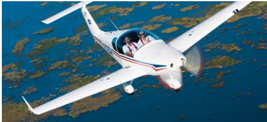
A T-tail and winglets set the Dova Skylark apart from most S-LSA; it's the only ready-to-fly LSA sporting both such features. The swept winglets are intended to convert wingtip vortices into lift, a concept proven on faster aircraft.
